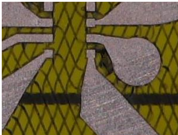
Figure 8: Double-sided flexible sample detail (50%) processed with ProtoLaser R4 (hatch & delamination)
