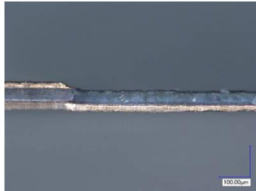
Figure 31: Fully removed copper after second pass
