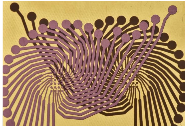
Figure 20: Double-sided Pyralux CG 185018 (18 µm Cu, 50 µm dielectric)
