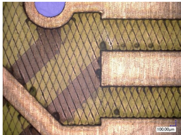
Figure 5: Double-sided flexible sample detail (100x) processed with ProtoLaser U4
