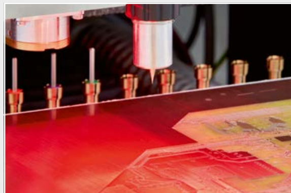
Double-sided FR4 material processed with LPKF ProtoMat S104
