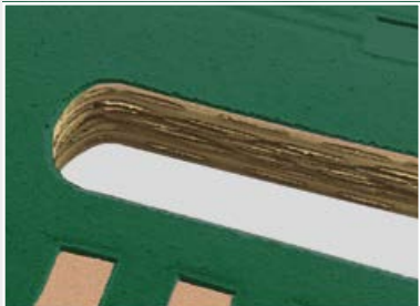
Cutting of mounting holes
