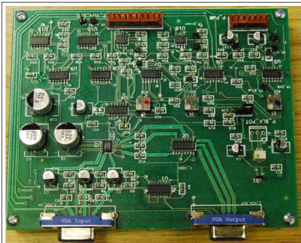
**Figure 2: Many designers prototype boards using PCB mills to ensure that designs are accurate before initiating high volume runs. Verifying the logical schematic of complex designs as hardware prototypes significantly reduces the risk of having costly and time-consuming errors arise in the field.**
