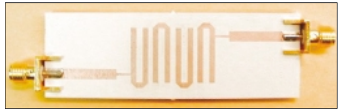
▲ Figure 6. Photo of the completed filter.
