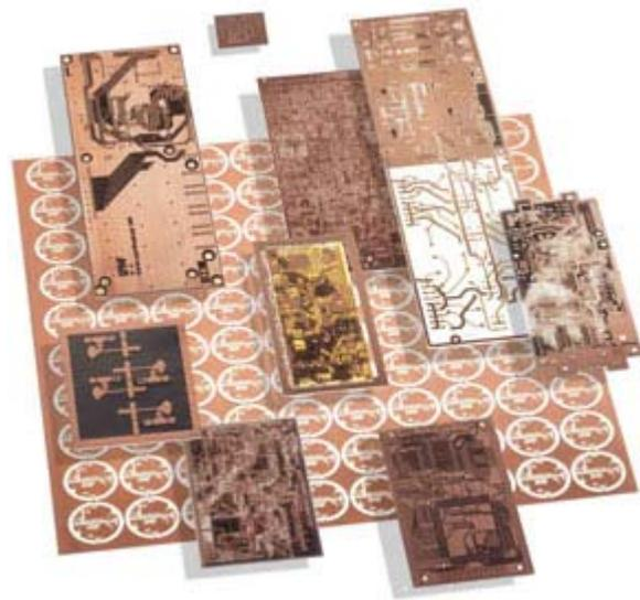
Mechanically milled circuit boards.
