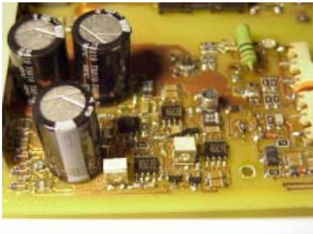
*Fig. 1: Milled and Populated Prototype Board*
