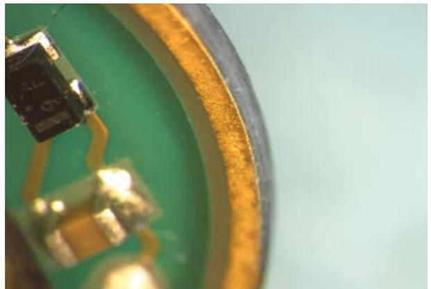
High quality UV laser depaneling ensures clean cutting channel side walls. Compared to  $\text{CO}_2$  laser processing, carbonization is virtually eliminated, increasing the breakthrough voltage threshold.
