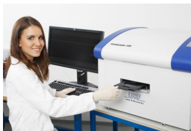
Compact and powerful: The LPKF ProtoLaser LDI exposes resists with structures down to the micron range
