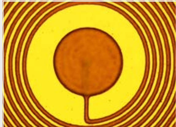
Processing stretchable flex PCB for wearables, deep engraving of PI for microfluidics
